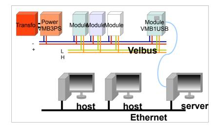
How it works ? The server application start the connexion to Velbus trhough VMB1USB (or VMB1RS for old PC). This application needs to know the COM port and on wich Ethernet port it has to wait client.
